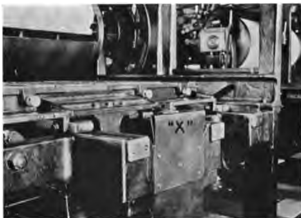
Fig. 4. Guard ("X") for Crushing Action at Rear of Miehle Press.‡
